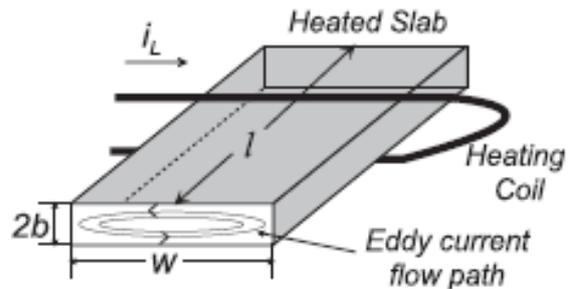
Figure 2. Model of slab for one turn coil.
