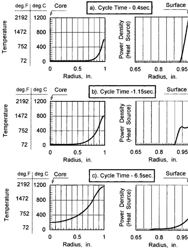
**Fig. 2.11** Interrelationship among heating time, power density, and hardened depth. Source: Ref 6
